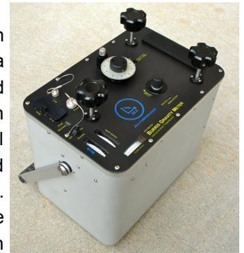
Each Burriss Gravity Meter™ is built around a handmade, metal, zero-length spring. ZLS springs have extremely low hysteresis and drift rates. When new, ZLS springs drift approximately 1.0 mGals per month after aging and when mature, drift less than 0.3 mGals per month. Data have shown that the spring's drift rate improves with age.
